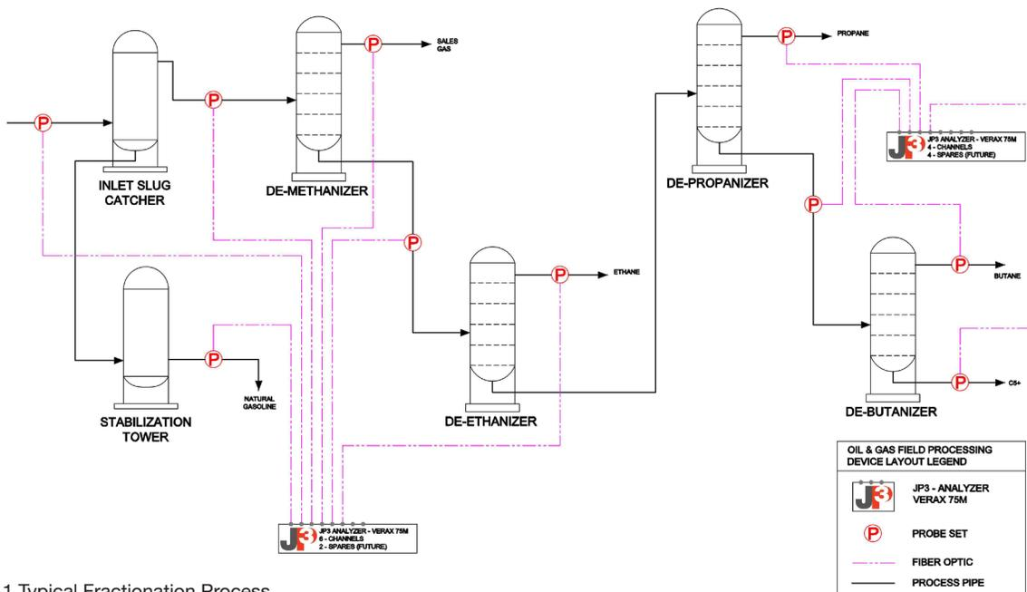
Fig.1 Typical Fractionation Process
